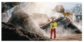
The material is placed in large piles, where microorganisms begin to break it down and heat up the piles to very high temperatures.
